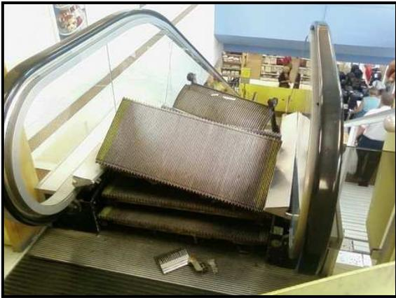
*The catastrophic failure of this escalator was investigated by the Inspectorate*
