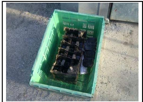
*The top of this lorry battery exploded whilst it was under charge, resulting in injuries to an engineer's face and eyes*
